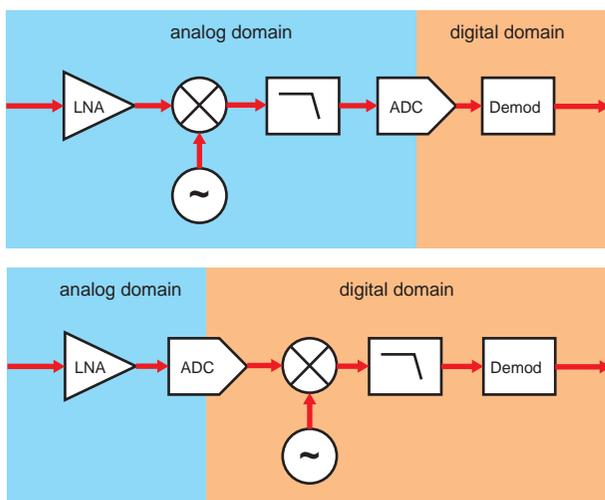
**Fig. 1: Conventional satellite tuner with superheterodyne receiver (top) compared with a next-generation satellite tuner with full-band capture (bottom)**
