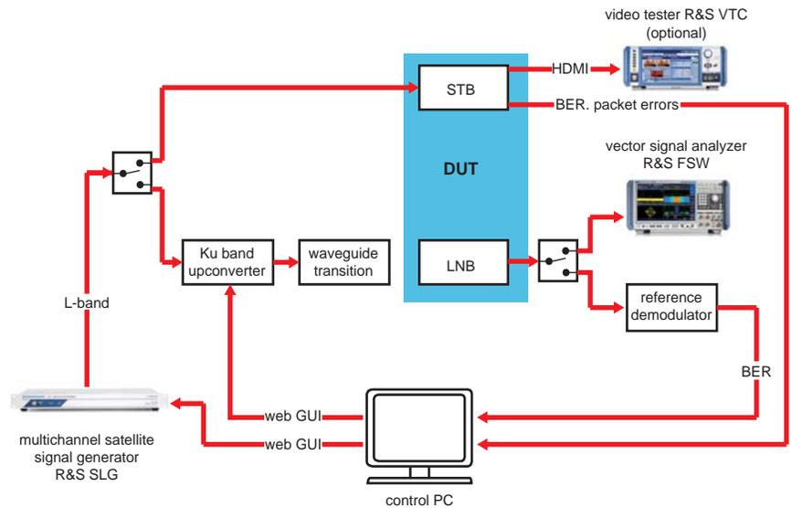
**Fig. 5: System for testing set-top boxes (STB) or LNBs with load profiles**
