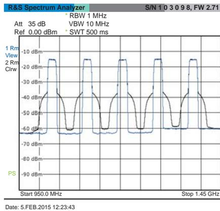
**Fig 6: Selective degradation of the signal quality in a transponder occupancy with phase noise. To highlight the effect, only every third transponder was activated.**
